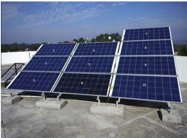
Fig. 1. 1 kW p multi-crystalline Si PV experimental setup at CEEE, NIT Hamirpur.
